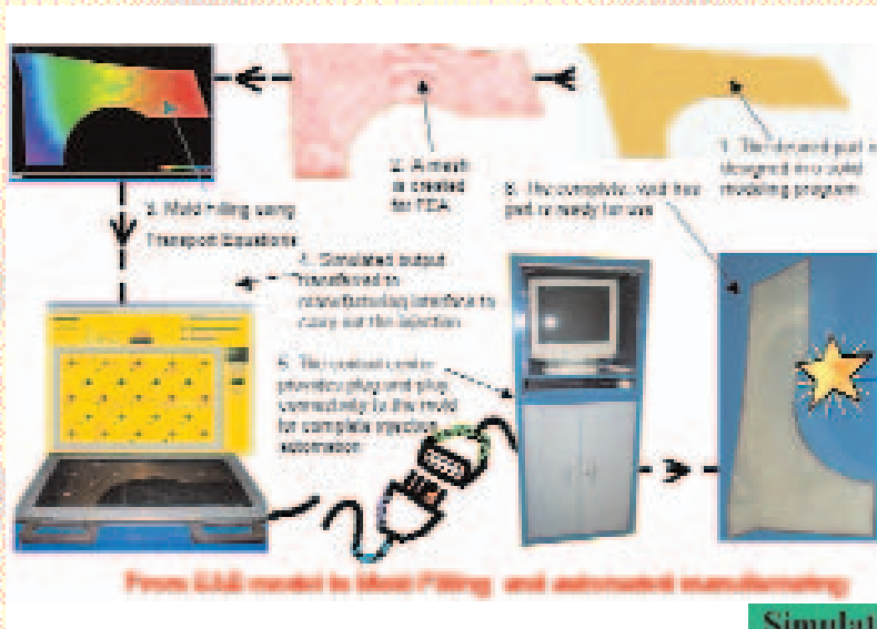
From Solid Modeling to Simulation of Mold Filling to Automated Control of the Process
